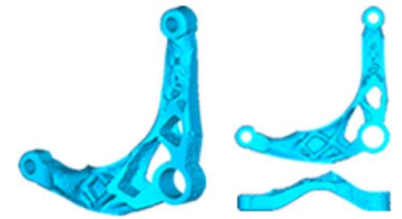
Result Shape by Die Drawing Topology Optimization
