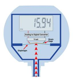
Digital pressure gage with a piezoelectric element and diaphragm (1)
