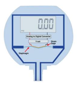
Digital pressure gage with strain gages and diaphragm (3)
