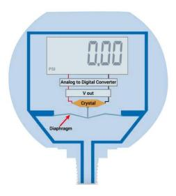
Digital pressure gage with a piezoelectric element and diaphragm (2)
